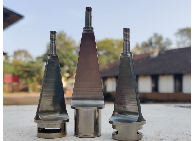
ARB blades, a part of the anti-roll bar assembly
