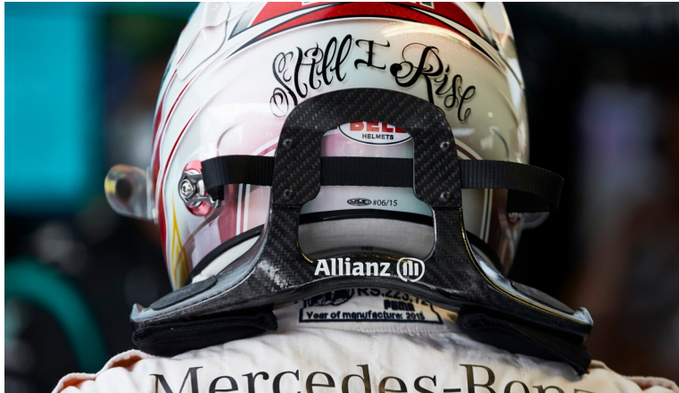
The HANS device integrated with helmets of all F1 drivers
